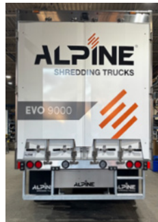
Strobe Lights, LED tail & reverse lights, lock-rod covers, rear bumper with step
